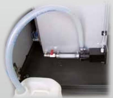
Built-in tank draining pump for used cooling medium.
